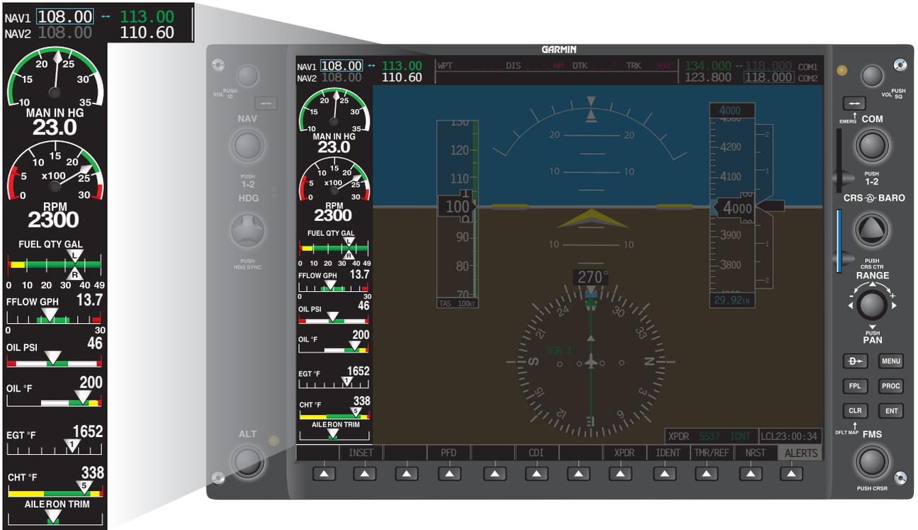
Figure 14-4. Powerplant instrumentation—fixed shaft turboprop engine.
