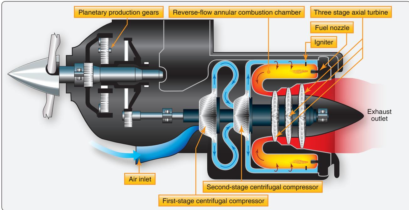
Figure 14-2. Fixed shaft turboprop engine.
