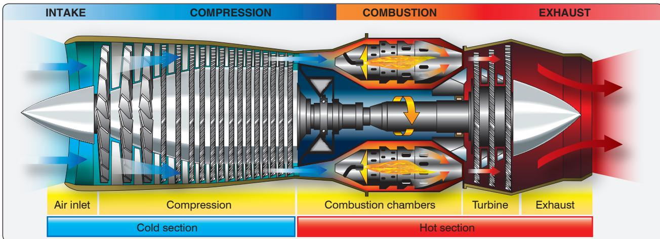
Figure 14-1. Basic components of a gas turbine engine.
