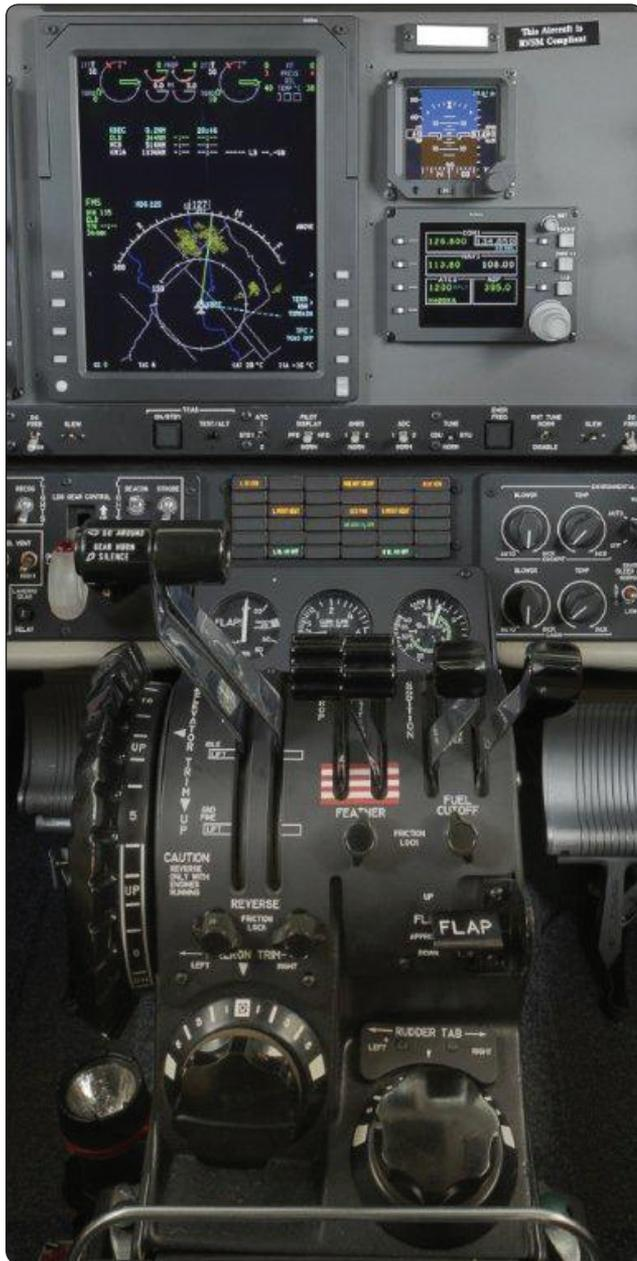
Figure 14-6. Powerplant controls—split shaft/free turbine engine.
