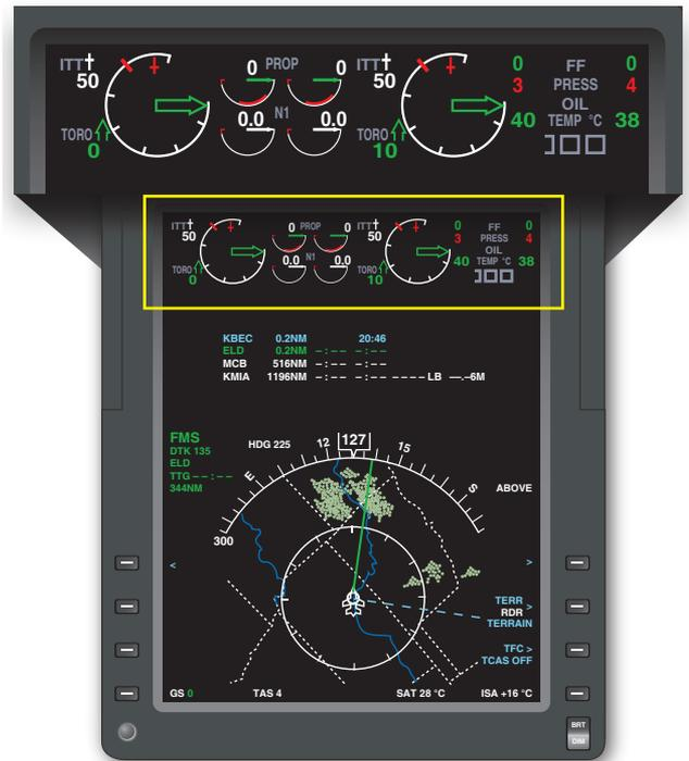
Figure 14-7. Engine instruments—split shaft/free turbine engine.
