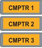
Illumination indicates that the control switch of the relevant computer is in the OFF or MAN position, or that the corresponding computer has failed (electrical power supply failure, internal failure or incorrect data).
