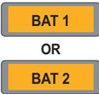
Illuminates to indicate that the corresponding battery is not connected to its bus.
