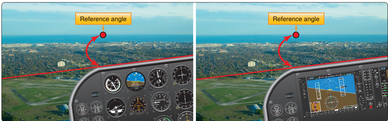
Figure 3-16. Visual reference for angle of bank.
