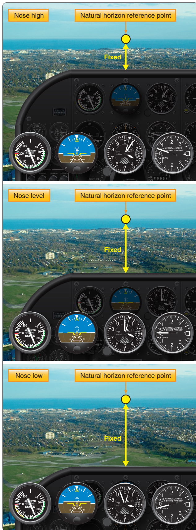
Figure 3-8. Nose reference for level flight.
