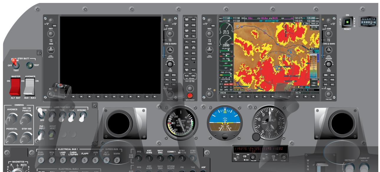
Figure 8-13. Multi-function display (MFD).
