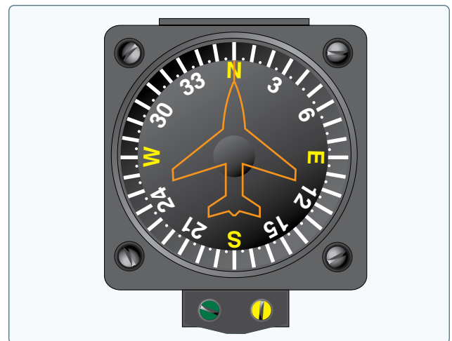
Figure 8-38. Vertical card magnetic compass.
