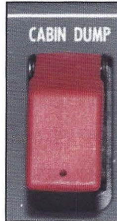
Figure 5-35: Cabin Dump Switch
