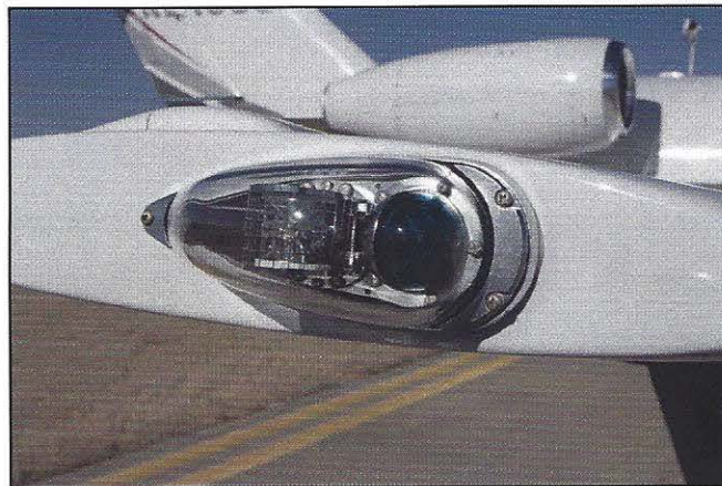
Figure 5-20: Wing Navigation Light
