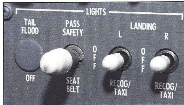
Figure 5-19: Light Switches (Landing and Advisory)
