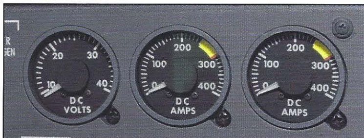
Figure 5-9: DC Power Indicators
