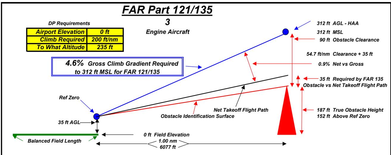
As you can see, simply adding .9% would have resulted in only 4.2% instead of the required 4.6%.
