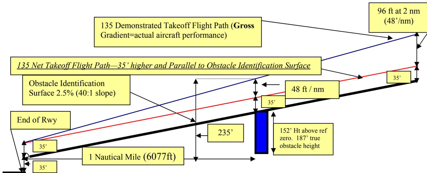
**The bottom line is this:** If there is an obstacle departure procedure and you cannot avoid obstacles visually, compute your max takeoff weight based upon the gross gradient required to fly that procedure either 91 or 135. If no DP is published but there is a known obstacle of known height and distance (very rare!), use the obstacle clearance charts to determine the gross takeoff flight path required. The obstacle clearance charts satisfy both 91 and 135 requirements.
