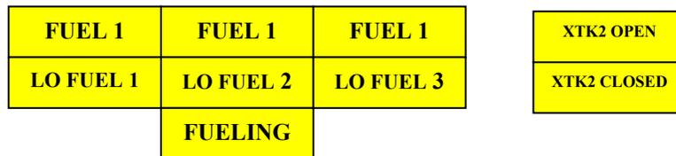
The **FUEL 1 2 3** lights illuminate when a pressure equal to or less than 4.6 psi is detected
