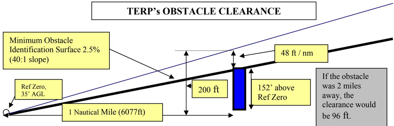
Transport Category Aircraft (FAR 25) have performance charts that allow you to calculate the one engine out steady gradients of climb you can expect under different density altitude and takeoff weight conditions. The steady gradient of climb (*called gross climb gradient*) is what the aircraft has demonstrated it will do if flown at  $V_2$  (for the second segment climb portion) at the appropriate takeoff weight by a pilot of average skill (just like every other performance chart).
