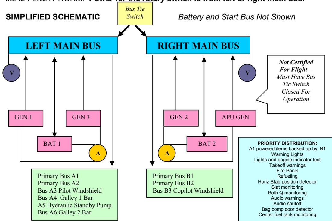
**Fault panel is “A1” bus powered backed up by B1. Gear down indicators are “B1” bus powered backed up by “A1”.**
