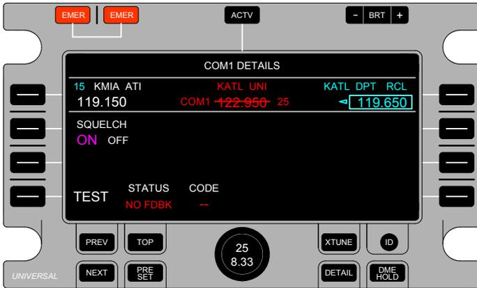
Active ATC feedback failure results in similar indications as the COM feedback failure. Whenever the RCU does not receive feedback from the active transponder, the RCU displays a Transponder Type Indicator (the active commanded Code dashed-out and the set Mode in red).
