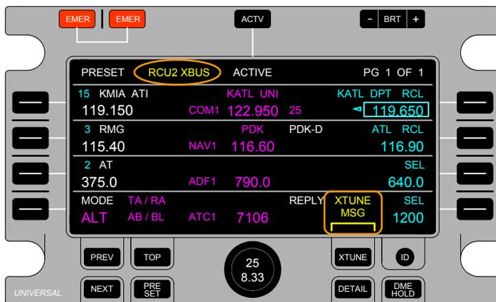
**NOTE:** The XTUNE MSG annunciator is displayed in-lieu of transponder FLIGHT-ID and ADS-B annunciators and annunciators in that field are not displayed until the XTUNE MSG annunciator is acknowledged / removed.
