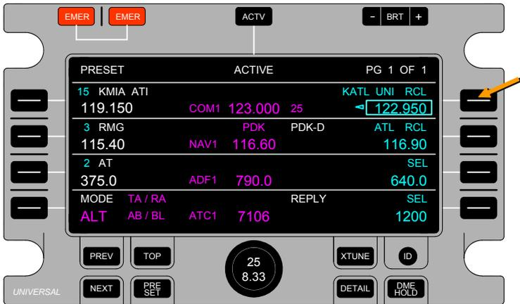
The frequency in the RCL/SEL column can be changed if needed. Once the frequency is changed, it will be labeled SEL (Selected).
