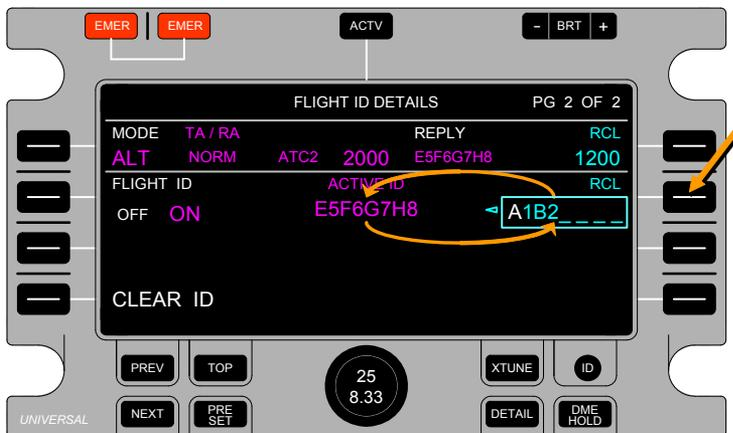
While the select box is located on the Standby Flight ID, pressing the associated LSK will activate the Standby Flight ID. The last Flight ID is now stored as the RCL Flight ID in the Recall/Select column.
