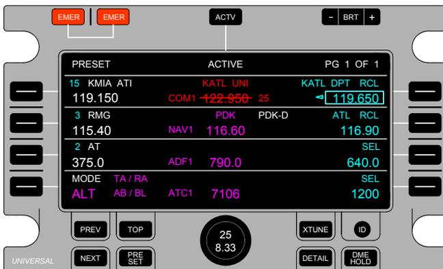
On the radio Details Page, the RCU indicates NO FDBK under STATUS and displays radio control option active setting(s) that are normally fed-back to the RCU from the radio all in red. In the following example, the COM Details Page is selected and the RCU is indicating it is not receiving COM radio feedback.
