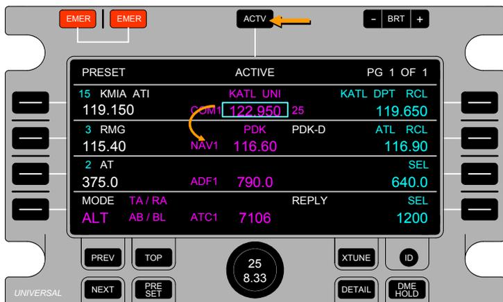
With each subsequent press of the ACTV Key, the Select Box will move down the Active Column to the next selection. At any of these selections (Active COM, Active NAV, Active ADF, or Active TCAS/ATC) frequencies can be tuned in the same manner described for Active COM Frequency.
