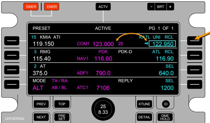
Once the Active and Selected frequencies are swapped, the frequency in the RCL/SEL column will be labeled RCL. If needed, the flight crew can switch the frequencies back by pressing LSK [1R].
