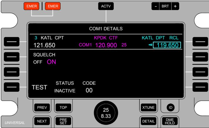
When LSK [2L] is pressed, a cyan Select Box appears around the Squelch ON OFF states. Squelch is ON, as indicated by the large magenta text. OFF is available as indicated by the small white text.
