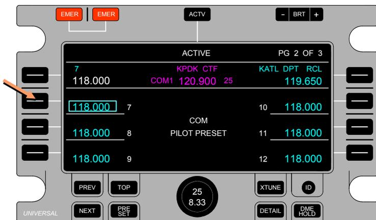
With the desired Pilot-Defined Preset Frequency selected, the frequency can be edited by rotating the Select Knob. The Outer Ring changes the left-hand digits (before the decimal point) and the Inner Knob changes the right-hand digits (after the decimal point). If the field is empty, the lowest possible radio frequency displays after the first rotation detent of the Select Knob. Continuous or subsequent rotations increment the desired Pilot-Defined Preset Frequency.
