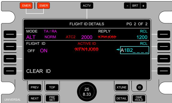
The active Flight ID can be directly edited by using the ACTV Key to move the Select Box around the active Flight ID.
