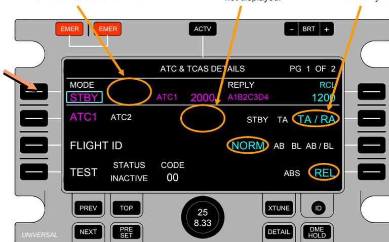
The Select Box will appear around the Active Transponder Side Select field whenever the ATC Details Page is selected. The active transponder side selection is available only on the ATC Details Page.
