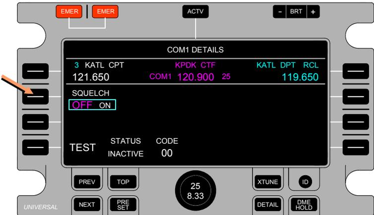
The other method of changing States is by turning either the Inner Knob or the Outer Ring one detent CW will select the next available State.
