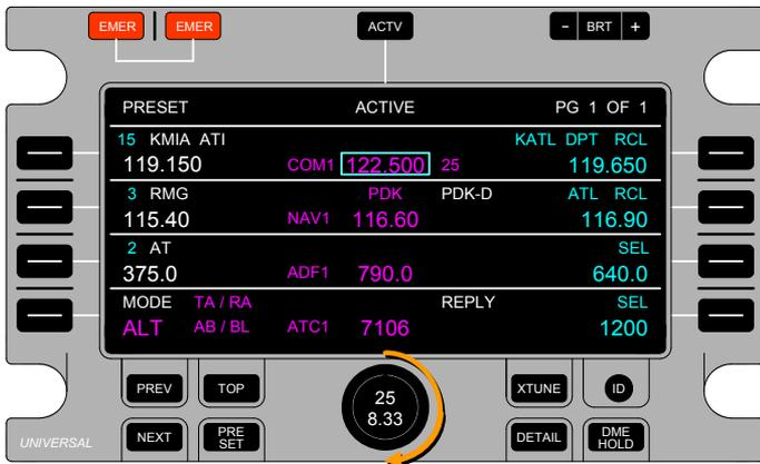
When the Select Box is moved to the Active COM frequency, pressing the ACTV Key again will move the Select Box down to the Active NAV Radio frequency. The NAV Radio frequency can now be direct-tuned with the Select Knob as previously described with the COM frequency.
