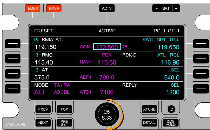
Two seconds after the COM radio fails to tune the new frequency, the RCU will then display the COM Radio Type Identifier and COM frequency as fed-back to the RCU in red and dashed-out.
