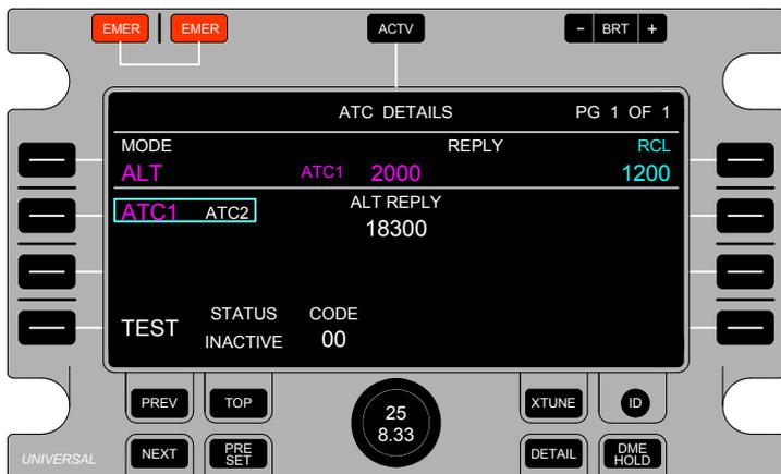
For dual RCU installations, both RCUs provide control of the active transponder and implement the last set code, regardless of installation side.
