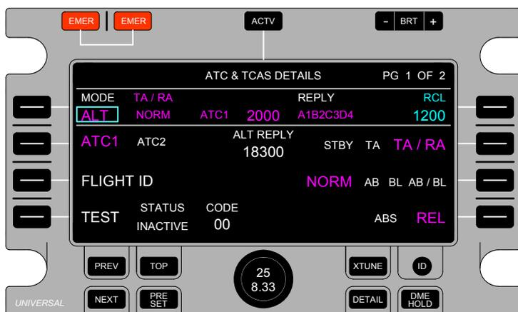
The Transponder/TCAS Details Page setup has some differences from the COM, NAV, and ADF radio Details Pages.
