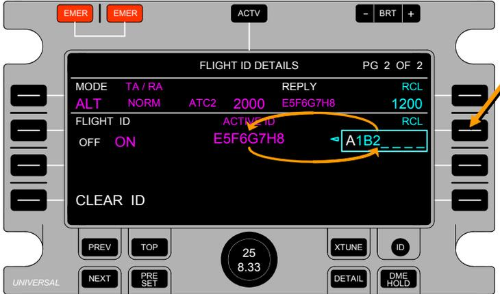
The RCU will display the new active ID for two seconds after it is first commanded, and after that it shows the ID as fed back from the transponder. Failure to receive the same ID as commanded will result in the RCU displaying the fed-back ID in red and dashed out. ATC RTI and the ACTIVE ID status indicators are also shown in red.
