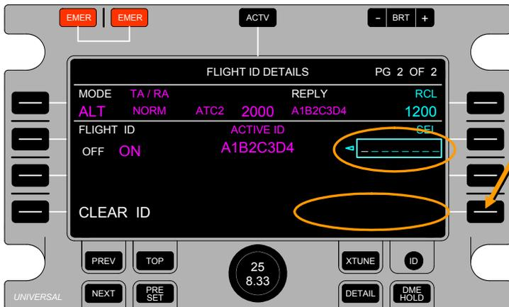
The RCU also has a Flight ID clearing function that can be enabled during configuration. This feature will clear the Active Flight ID when the RCU is powered up and W.O.W. is enabled, during configuration, and set.
