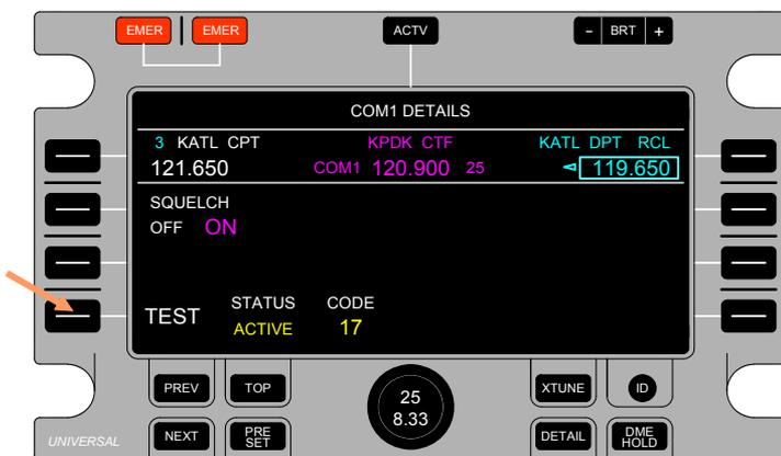
**NOTE:** When the radio has completed the self-test, the RCU will change the Test Status indication from ACTIVE to INACTIVE (even if LSK [4L] is still being pressed). This allows the person initiating the test to see that it is complete.
