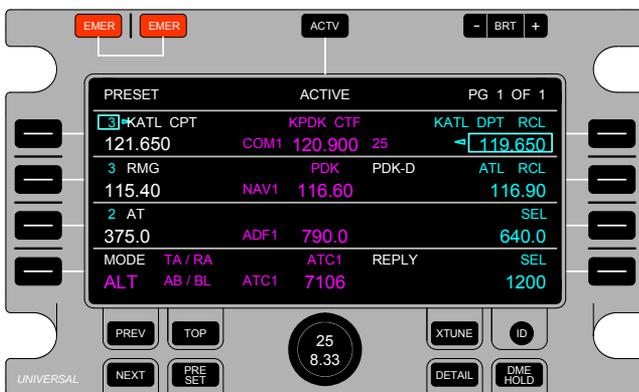
When the PRESET Key is pressed, the RCU will display the COM Preset Page 2.
