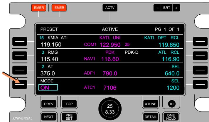
Also, the Select Knob can be used to change Transponder Modes (one increment per knob detent). The example below shows the Transponder Mode when the Select Knob is turned to the next detent.
