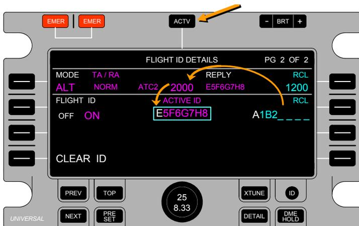
Use the Select Knob to set the Flight ID. The last commanded Flight ID is retained in the Recall column and will not change until the Select Box has been moved away from the active Flight ID position.
