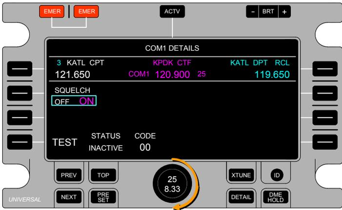
There is no wrapping to the leftmost State when the most rightward State is selected. Likewise, turning either the Inner Knob or the Outer Ring one detent CCW will select the next-leftward available State, with no wrapping.
