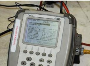
ADS-B ground testing equipment, as shown above, can verify all parameters are correct after an ADS-B installation. Once your equipment is installed, be sure to <u>find out if your equipment is</u> working properly.
