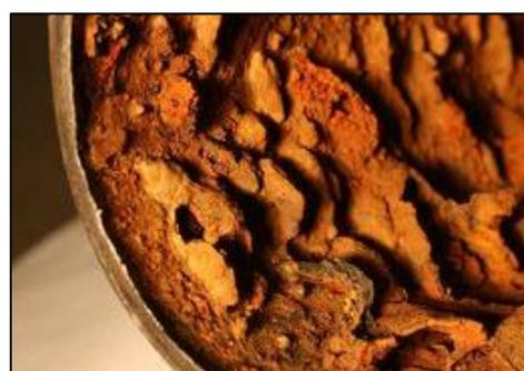
There are several corrosion mechanisms in amine units. The most common mechanisms are CO<sub>2</sub> and H<sub>2</sub>S induced corrosion. In some cases, the process might also experience ionic solvent corrosion when heat stable salts concentration is high. Additional corrosion pathways can also take place depending on the process conditions and the amine solvent type.
