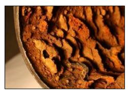
There are several corrosion mechanisms in amine units. The most common mechanisms are CO<sub>2</sub> and H<sub>2</sub>S induced corrosion. In some cases, the process might also experience ionic solvent corrosion when heat stable salts concentration is high. Additional corrosion pathways can also take place depending on the process conditions and the amine solvent type.
