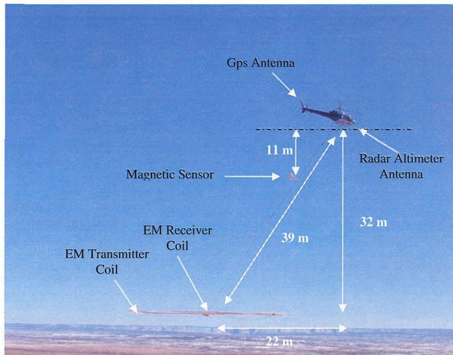
**Figure 6 - Conventional VTEM-M system configuration**
