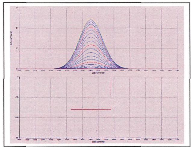
Figure C-12: B-Field response of a deep horizontal thin plate. Depth=200 m, CT=20 S. The EM response is normalized by the dipole moment.
