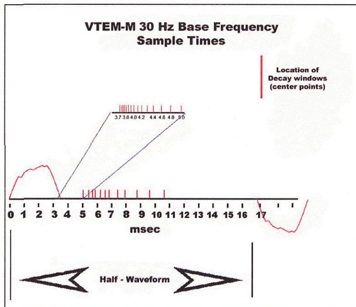
Figure 5 – VTEM-M Waveform & Sample Times
