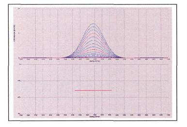
Figure C-11: dB/dt response of a deep horizontal thin plate. Depth=200 m, CT=20 S. The EM response is normalized by the dipole moment and the Rx area.
