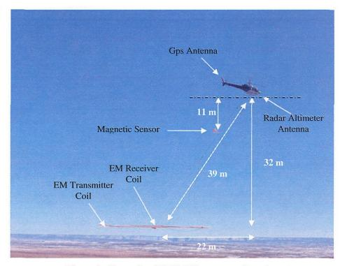
Figure 6 - Conventional VTEM-M system configuration
