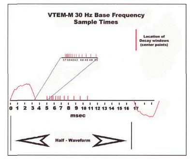
Figure 5 – VTEM-M Waveform & Sample Times
