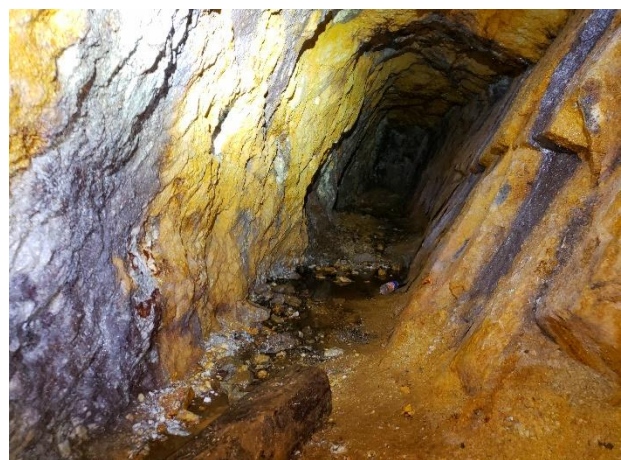
Left Photo: Inside the adit at the 40-meter mark. Boards cover flooded winze. Right Photo: Left crosscut, sericitized zone.
