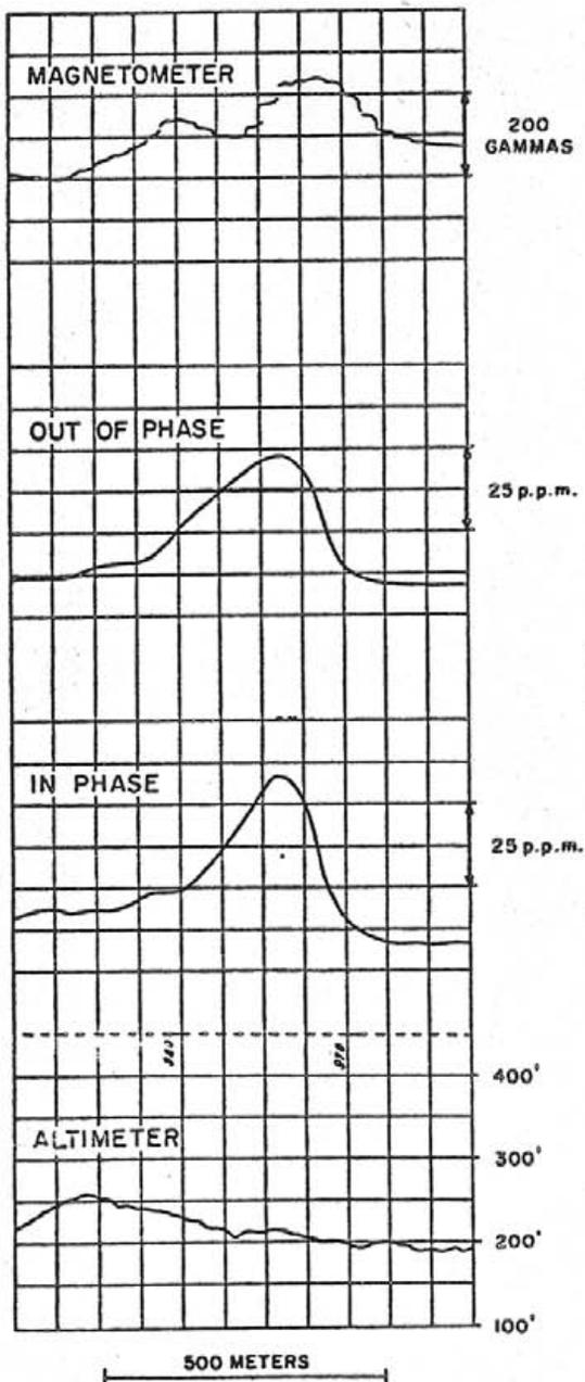
Figure 4: HEM-801 and magnetometer data
