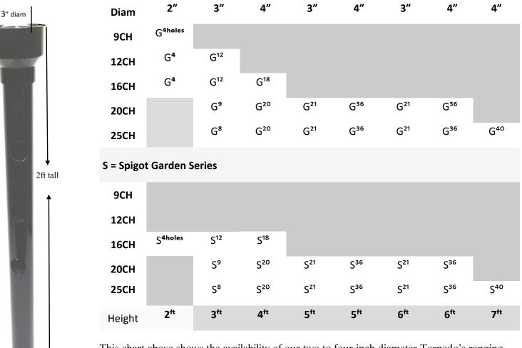
This chart above shows the availability of our two to four inch diameter Torpedo's ranging from two to six feet in height. The subscript denotes the number of openings in each Torpedo. Each hole is  $1\frac{1}{2}$  inches in diameter.
