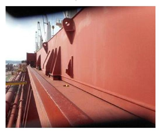
purpose is to transfer the cover's weight to the ship's hull while allowing for relative movement between the cover and the hatch coaming caused by hull flexing whilst the vessel is at sea.
