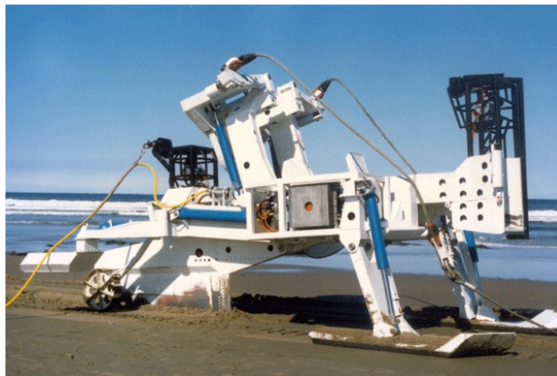
Figure 22 - A Cable Plough
