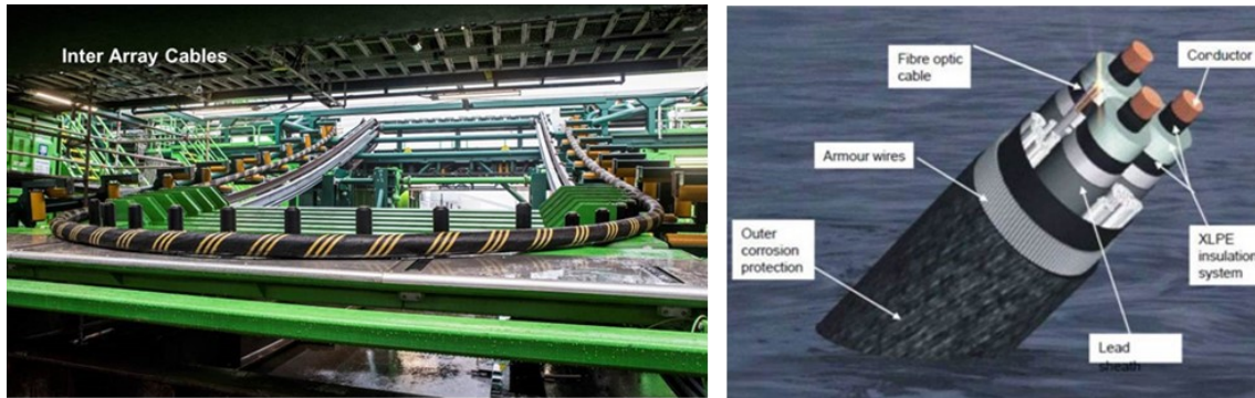
Figure 25 - The Inter-array cables
