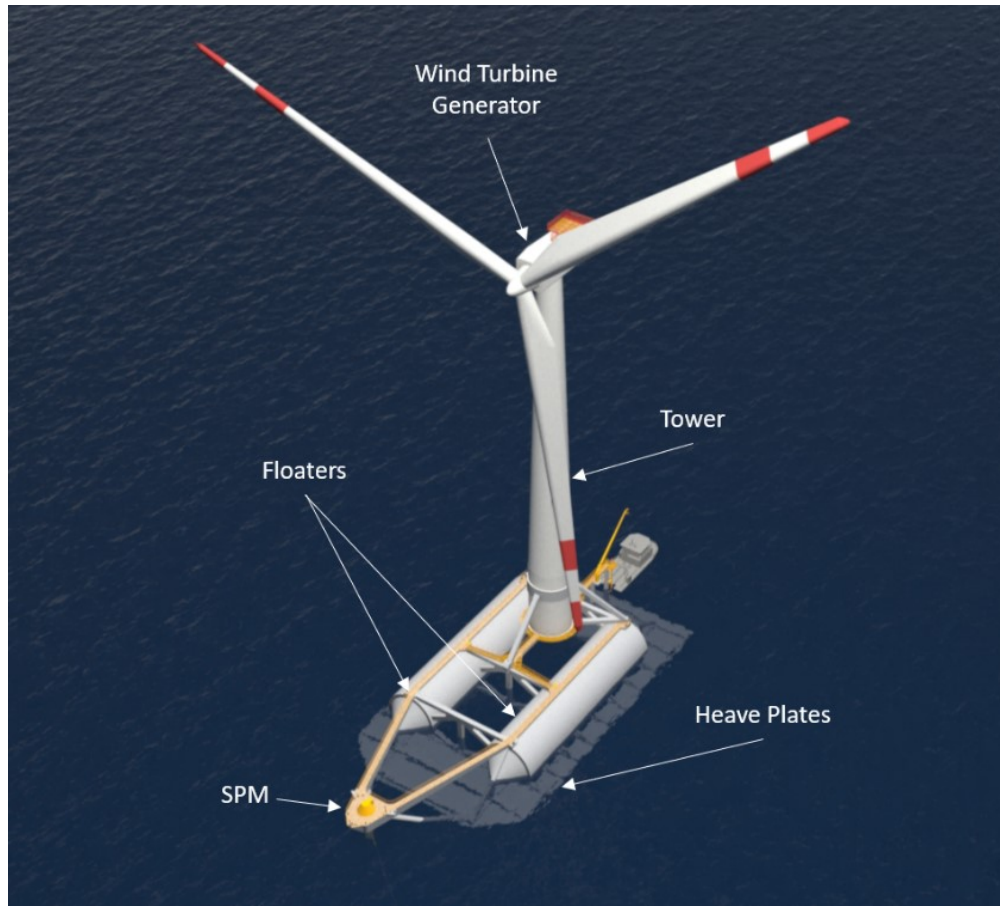
Figure 7 - SATH Floating Barge Technology General Layout
