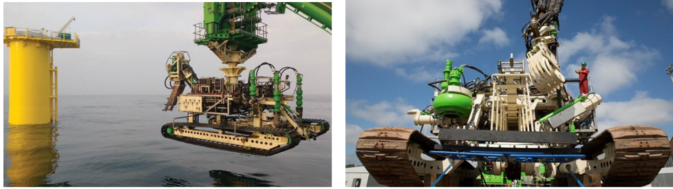
Figure 21 - A Jet Trenching ROV (DEME trenching Tool CBT1100)
