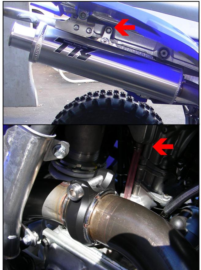
*Locate the top mounting bracket on the silencer body, and swing it up 90 degrees from the silencer. Using one of the stock silencer mounting bolts, run this bolt in the silencer mount and into the frame finger tight.*
