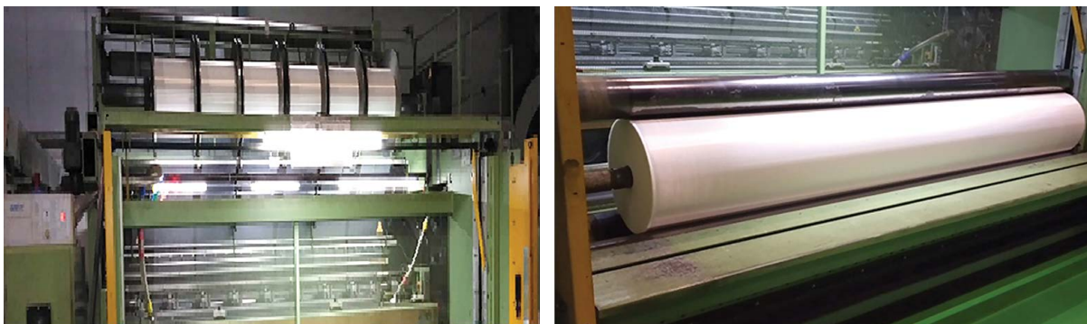
Figure 31. Knitting of the Polyester Fabric
