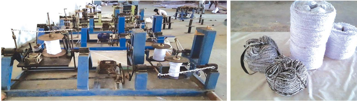
Figure 42. Fabrication of High Strength Ropes from the By-Products of the Flex Banners
