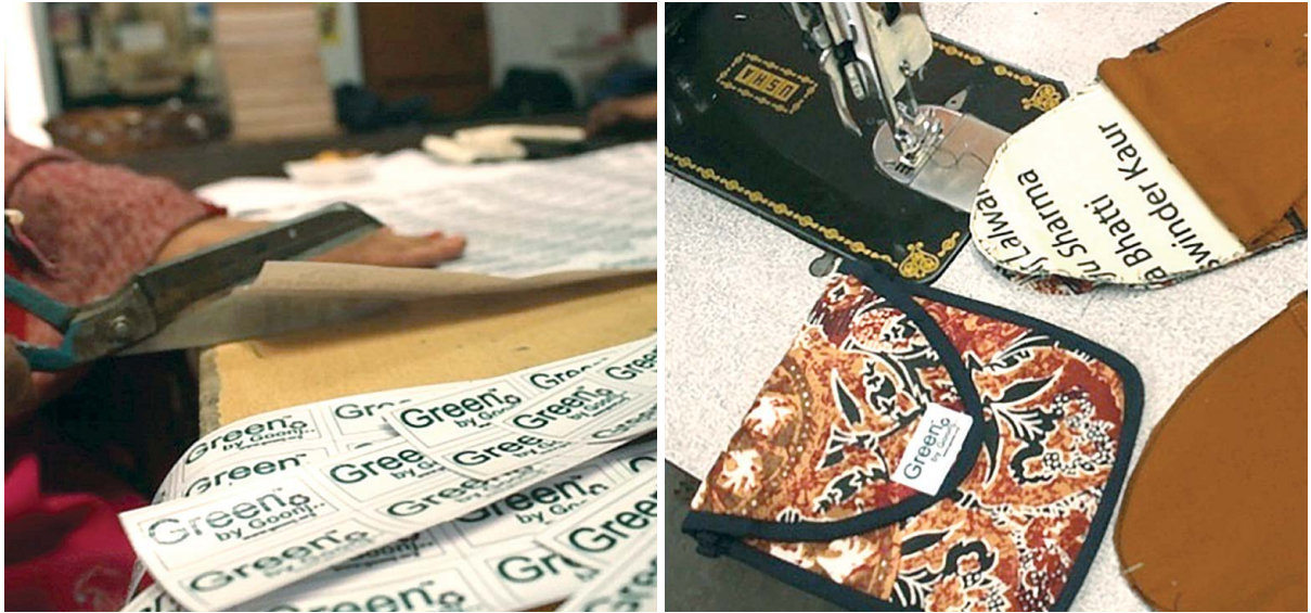
Figure 37. Fabrication of Pouches from the Disposed Flex Banners [23]
