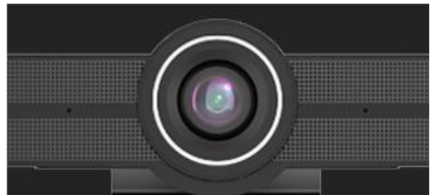
Full circled WHITE light turns on/turns off signifies camera is opened/closed
