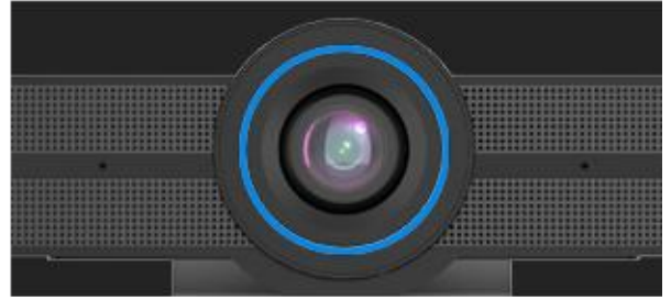
Full circled BLUE light signifies camera & remote control are paired
