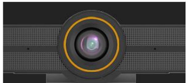
Full circled ORANGE light flashed / disappear, long press menu button on remote to enter into setting mode, press OK button, the flash light will disappear
