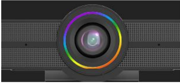
RAINBOW marquee running 3 seconds slowly, camera is powered on
