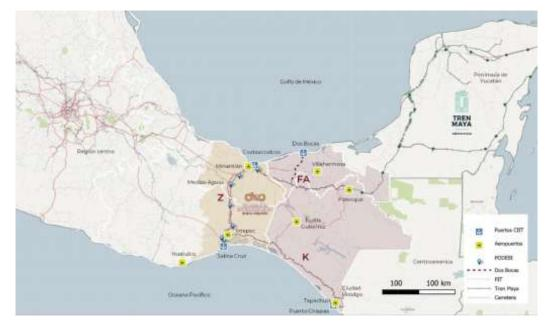
Undoubtedly, the train is the most important component, which in fact the president has dubbed the "spinal cord of the Interoceanic Corridor". Its principal railway is the transystem (Line Z) which connects the Gulf of Mexico with the Pacific Ocean, connecting the ports of Coatzacoalcos y Salina Cruz.
