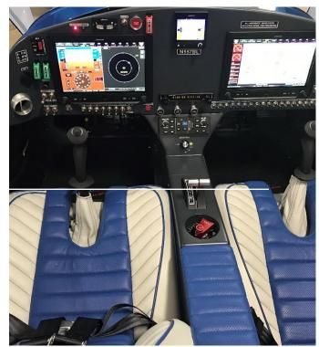
This Bristell 912iS Sport is equipped with dual G3X 10inch Touch Screens, a Back up G5, and a Val 2000 Certified ILS receiver. If the owner changes it to an ELS, it can be flown IFR in IMC.
