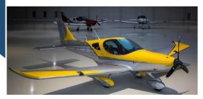
Bristells are constructed of tried-and-true aluminum. The aluminum is 6061 grade, the same as used on the space shuttle. Milan Bristela, the CEO and Aeronautical Engineer that designed Bristell, decided to use 4 grades of aluminum to keep the weight low. Carbon fiber is also used to save weight.
