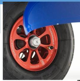
The Berringer Wheels and Brakes enhance Safety because they are anti-lock and anti skid. The bearings are sealed and last 7 years. The wheels do not need to be removed during the annual inspection reducing cost and wear.
