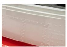
The 3400 rivet heads are filled with epoxy, sanded and painted to prevent corrosion and result in a professional looking aircraft.
