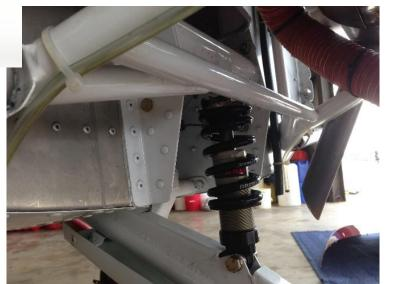
The nose wheel has dual shock absorbers. A center hydraulic cylinder and an outer steel coil spring.
