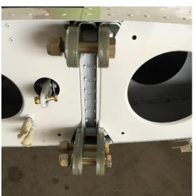
Massive wing bolts attach to the spar both forward and aft. All Bristells have a Vne of 157 KIAS. This is one strong airplane.
