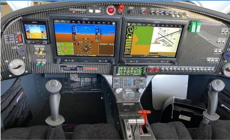
This panel has the FAA certified Garmin GNX375 receiver for GPS, LPV vertical guidance approaches for IFR flight in IMC with ADS-B in and out
