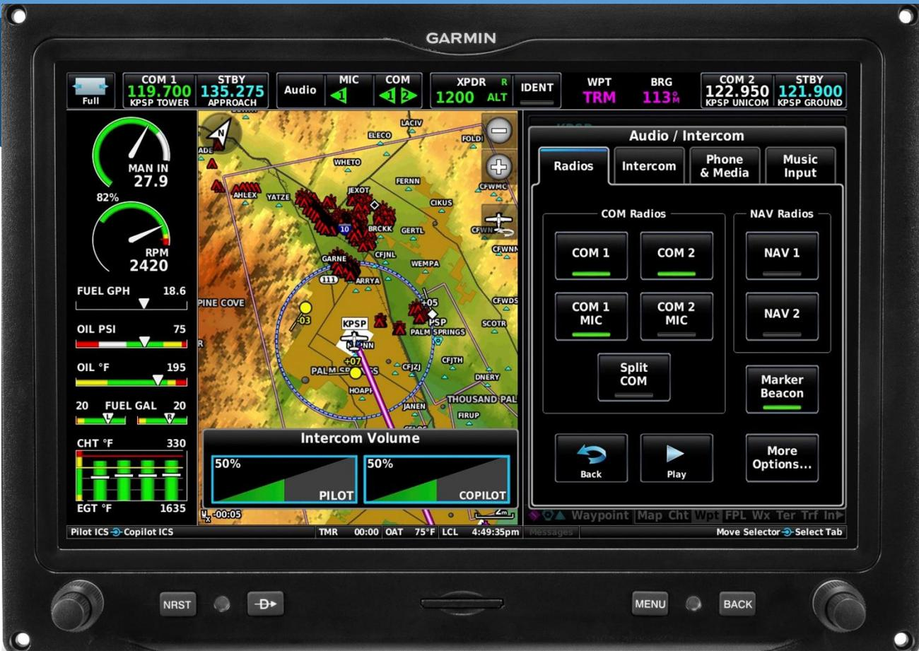
The Com is displayed in the upper left-hand corner. Touching the blue STBY box will place the STBY frequency in the Com 1 Box.
