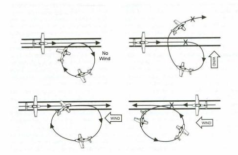
Draw an imaginary line from the point where the wind drift circle began to the point where the airplane ended up when the wind drift circle was completed.
