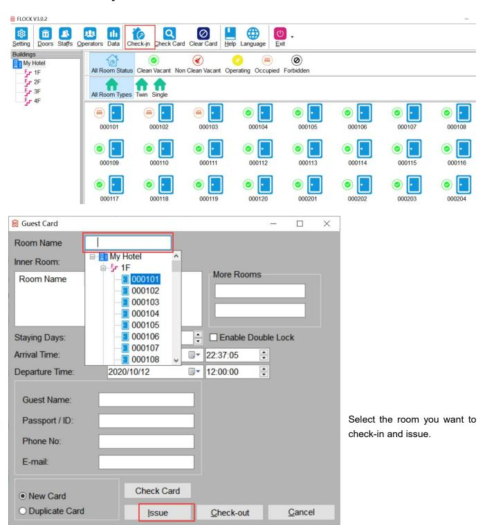
Guest card is done, then take this card to the corresponding room, try to open the lock. Green light and 1 beep, motor run from the lock, so you can push the handle.
