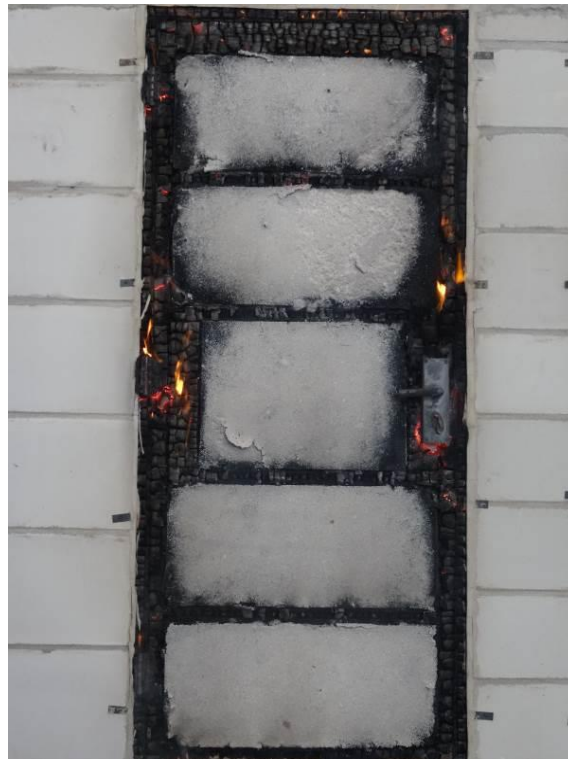
Fig. 10 – Exposed Side after 60 Minutes
