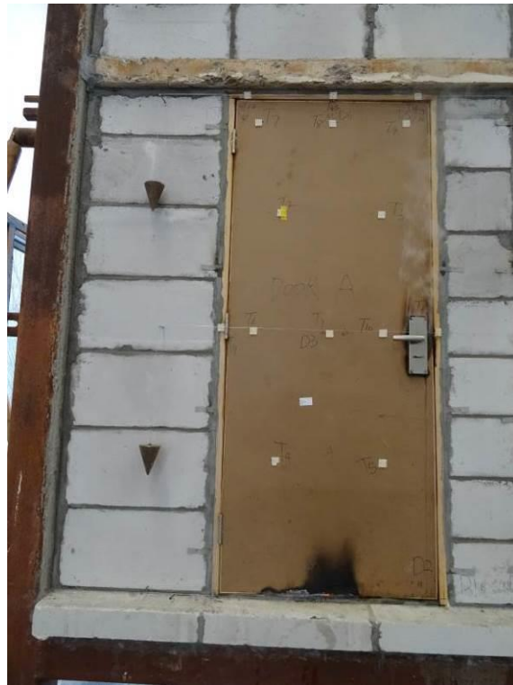
Fig. 7 – Unexposed Side after 60 Minutes
