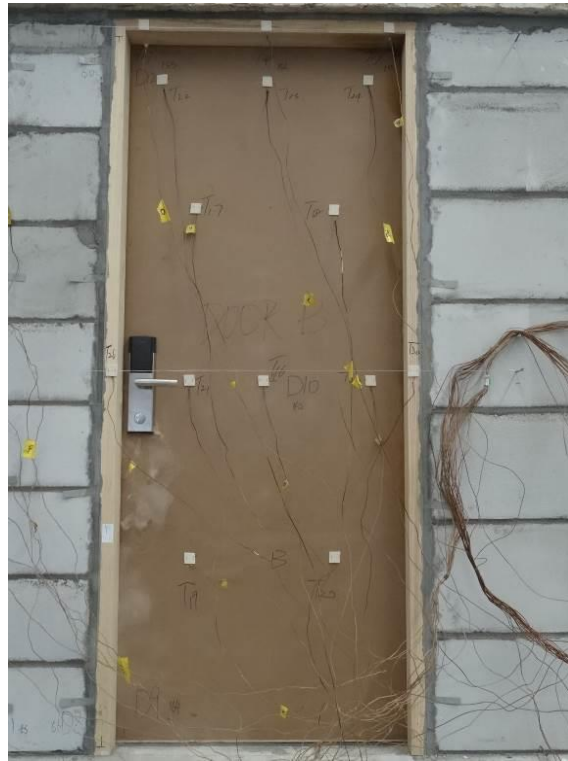
Fig. 3 – Unexposed Side after 10 Minutes
