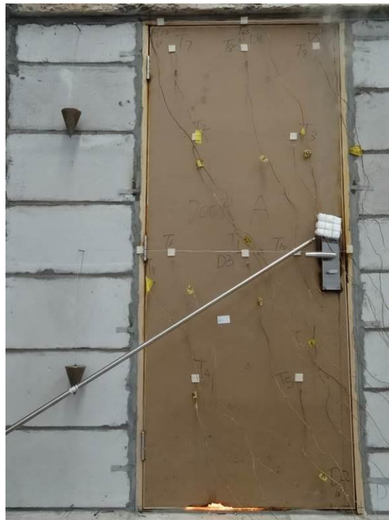
Fig. 6 – Unexposed Side after 58 Minutes
