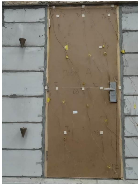
Fig. 4 – Unexposed Side after 20 Minutes
