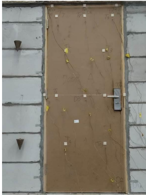
Fig. 5 – Unexposed Side after 30 Minutes
