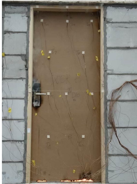
Fig. 9 – Unexposed Side after 60 Minutes
