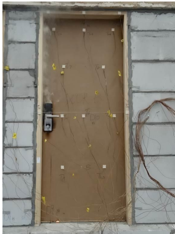
Fig. 6 – Unexposed Side after 51 Minutes
