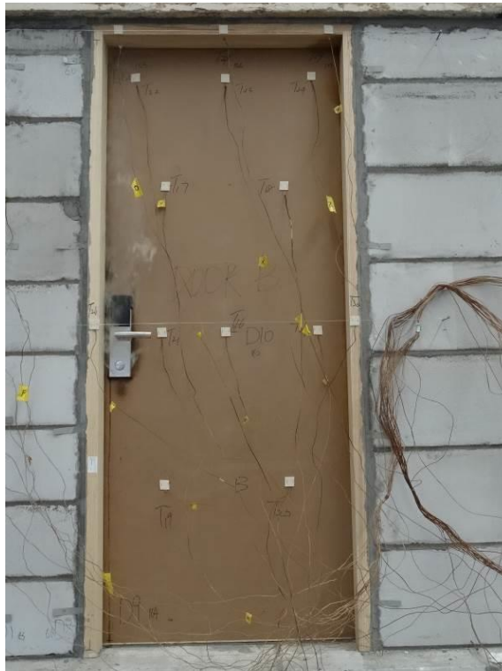
Fig. 4 – Unexposed Side after 20 Minutes
