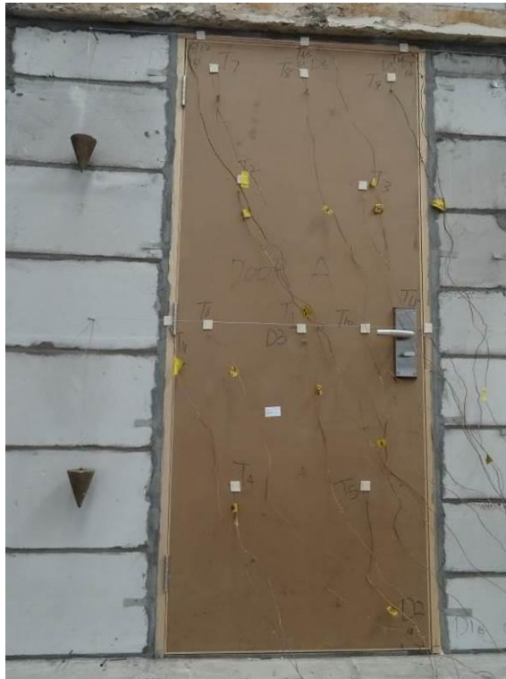
Fig. 1 – Unexposed Side Prior to the Fire Test
