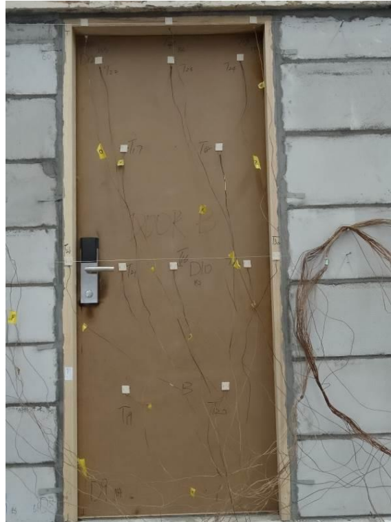
Fig. 5 – Unexposed Side after 30 Minutes
