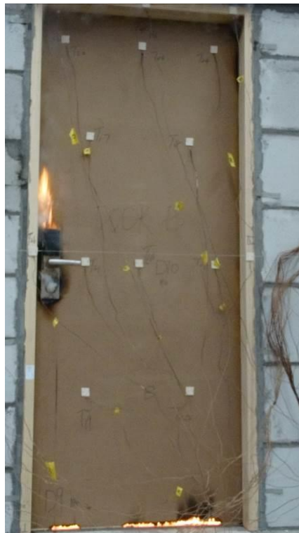
Fig. 8 – Unexposed Side after 59 Minutes
