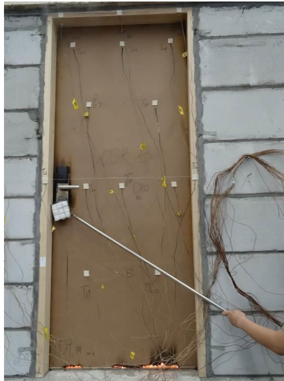
Fig. 7 – Unexposed Side after 57 Minutes
