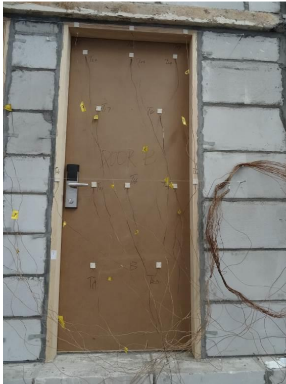
Fig. 1 – Unexposed Side Prior to the Fire Test
