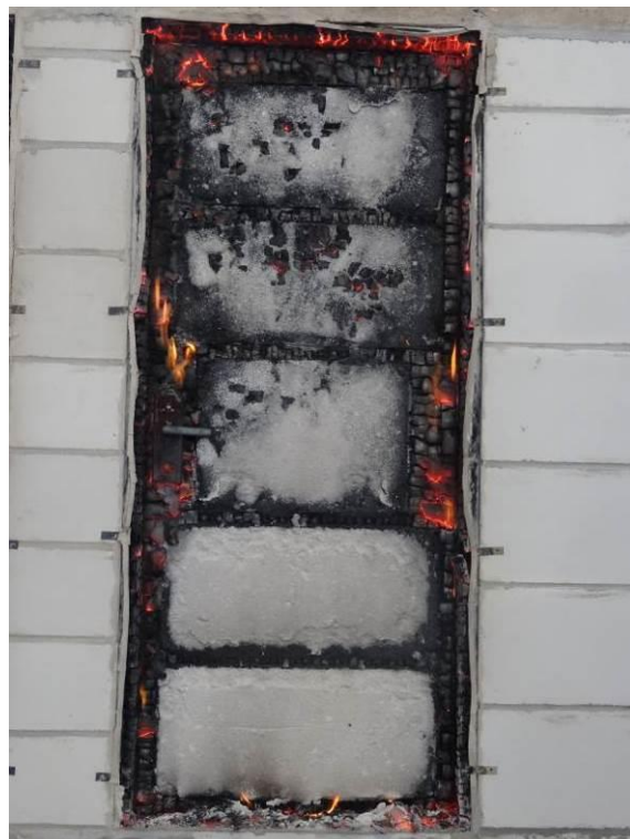
Fig. 8 – Exposed Side after 60 Minutes
