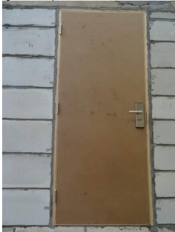
Fig. 2 – Exposed Side Prior to the Fire Test
