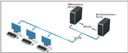
Be-Tech server interface with PM via RS-232, PMS terminal and PMS server share the Ethernet network. Encoders connect to the PMS terminal PC.
