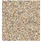
Gravel: Gravel is a budgetfriendly option that allows for excellent drainage, making it ideal for areas with heavy rainfall. While gravel driveways are easy to install, they require frequent maintenance to prevent ruts and keep the gravel in place.
