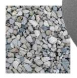
Crushed stone: Crushed stone driveways are similar to gravel but have a more uniform look. They offer excellent drainage and flexibility in design, though they can become uneven over time without regular upkeep.
