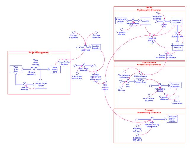
**Figure 4:** Expanding the rework cycle with installed capacity (produced by the project) to integrate project management with innovation and sustainability (Calderon-Tellez, 2022).
