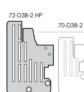
The 72-D3B-2 HP has a larger needle plate and 6 rows of feed dogs.
