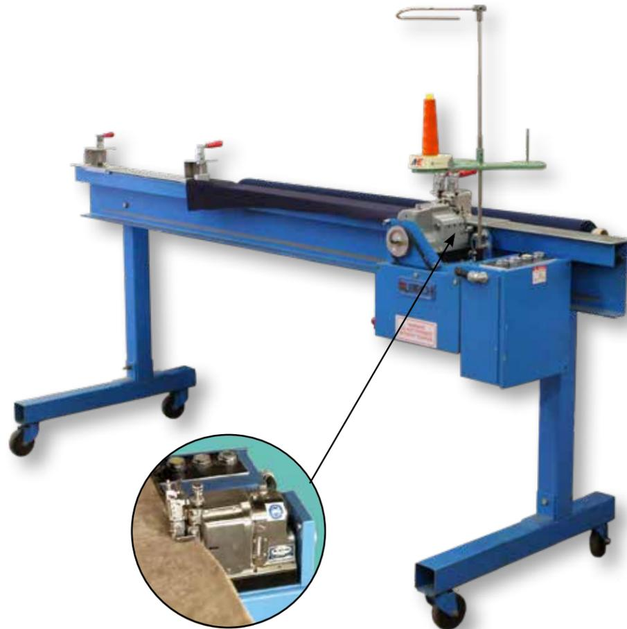
A railway system completely automates production, providing straighter and faster end-to-end seaming. The belts, pulleys, clutches, rack gear, and carriage wheels of older machines have been eliminated for simplified maintenance, saving time, material, and money.
