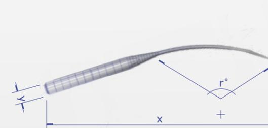
All Merrow needles are engineered to within one one-thousandth of an inch, and strict quality control measures during manufacture ensure that each needle is made to the same exacting standard.
