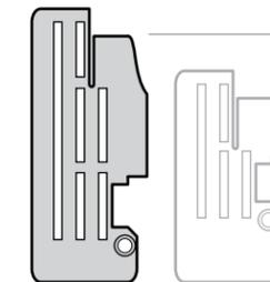
The 72-D3B-2 has a larger needle plate and additional feed dogs.
