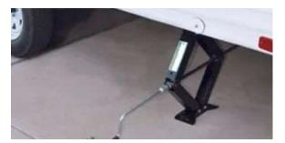
The driver and crank are inside of storage compart. All our campers have some version of this stabilizing jack. Using the tool provided, lower the jack to the ground. These need to be snug, but they are not made to lift the camper. It prevents the camper from moving as much when people are moving around inside.
