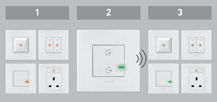
Once all wired devices are installed and the power is on, all LEDs will light up in red. Press the master switch in the centre and hold for 5 seconds.
