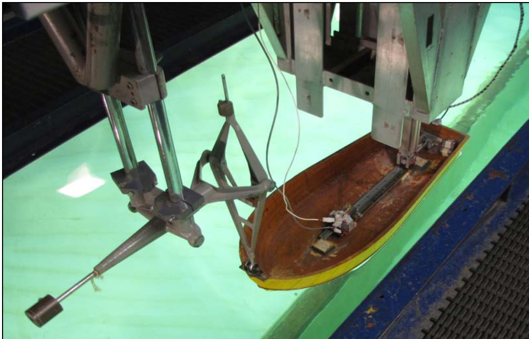
Figure 1. Series 62 Model No 4667-1 attached to MHL dynamometer
