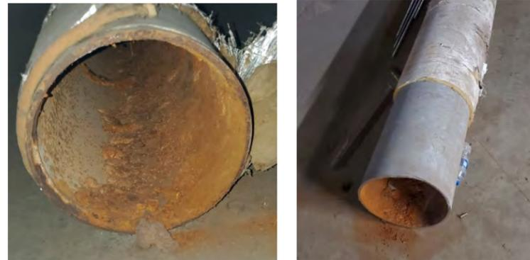
*Domestic water galvanized steel pipe corrosion*
