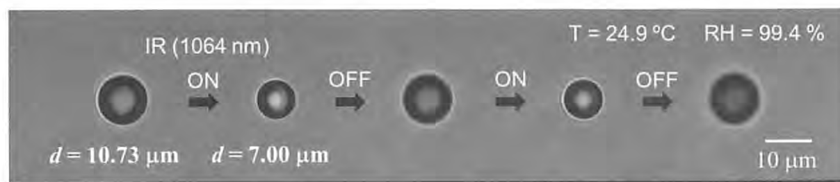
Fig. 1 Reversible size changes of the aqueous ammonium sulfate droplet in air upon switching on-off of IR laser irradiation.
