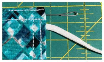
Nose Wire: Put a 22 gauge piece of wire in the casing. Bend both ends so it doesn't poke holes or people.
