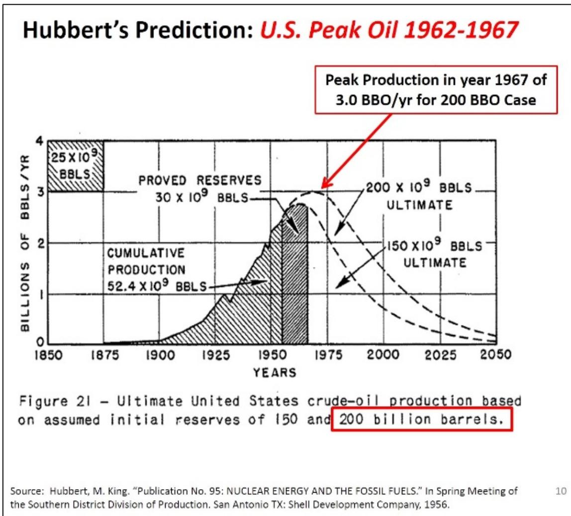
Figure 2 – Excerpt from Hubbert’s 1956 Paper (annotated)
