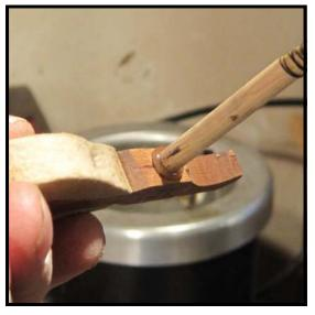
**Step 46:** Insert the hammer shank into the hole in the hammer molding, and swivel it back and forth to create a collar of glue as you push the shank in to the correct depth. Line up the two matching reference lines.
