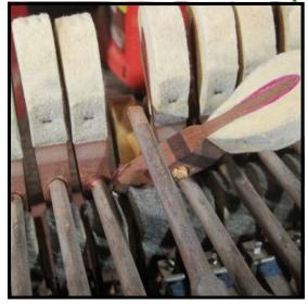
Note: This type of break necessitates either replacement of the shank, or splicing in with a segment of new shank. In the case of this particular piano, a new set of shanks and hammers were recommended and were slated to be installed at a future date. For the time being, however, repairing the piano to work was the order of the day. A simple splicing of several broken shanks was recommended as a temporary measure so that the piano might be played again.
