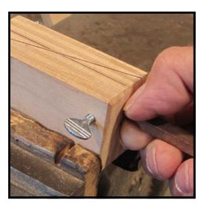
**Step 6:** Insert the flanged end of the hammer shank into the hole in the miter box up to where your fingers are holding it. Tighten the set screw on the end of the miter box closest to you.
