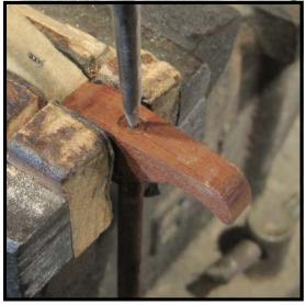
Step 29: Turning your attention to the corresponding hammer, place the hammer head in a leather or cork-lined vise as shown for removing the remaining portion of the broken shank. Use a sharp awl to mark the exact center of the top of the old shank.
