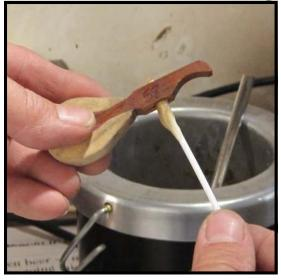
**Step 44:** Using a Q-Tip which you have dipped into your hot glue, swab the inside of the hammer shank hole in the molding of the hammer. Set the hammer down for a moment.
