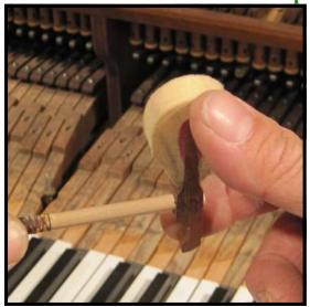
**Step 34:** Test the fit of the new spliced shank in the hole of the hammer head. It should be snug and tight, but not so tight that it ratchets (exhibits jumpiness when turned). If it is too tight, or if it can't be inserted into the hammer at all, the shank will either need to be reduced or knurled.
