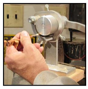
**Step 35b:** A more efficient knurling may be done with a production-type hammer shank knurler (Cat. No 217). Feed the end of the shank into the tool, turn the handle, and the job is done.
