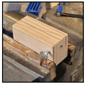
**Step 4:** Set up your hammer shank miter box in a heavy-duty vise for a more stable and accurate cut.
