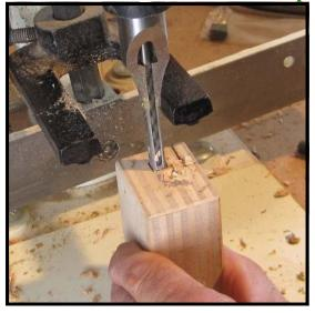
Cut the hole to the full depth, then widen it slightly by trimming another 1/32" or so from the sides with the chisel bit. Without just a bit of widening, most squared shanks will bind or refuse to go into the hole.
