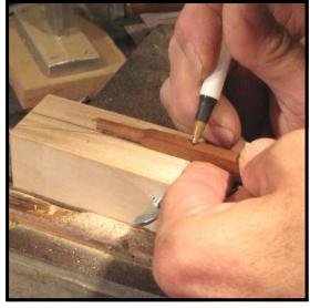
Now, repeat step 4. As an alternative to simply holding the shank at the correct point, you can also mark it with a pencil or pen.
