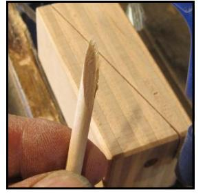
The matching gluing surface on the new splicer. One convenient thing about using the hammer shank miter box is that you never need to worry about the angle to cut. You will automatically have matching surfaces to work with.
