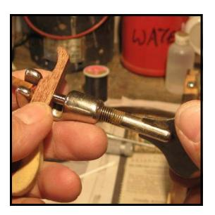
Step 30: Use a grand shank press (Cat. No. 131) to extract the old stub. Remove the hammer head from the vise, and place it in the press as shown with the point of the plunger lined up with the hole that you marked in the top of the shank. Carefully steam the glue joint where the shank is inserted, (avoid the felt) then begin turning the screw down.
