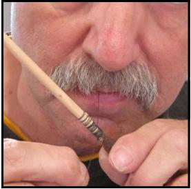
Step 21: Without releasing your hold on the end of the windings, take one end of the thread between your teeth again, and use your free hand to tie a simple knot. Cinch it up tight. (Again, for the purpose of getting everything in focus for the photo, the thread has been cut rather short. A little more length would make the job easier.) Keep the thumb of your left hand over the knot to prevent loosening.
