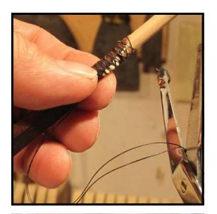
Step 20: Snip both ends of the thread, leaving about a foot or so of extra thread to work with (the photo shows the thread being cut rather short for the purpose of getting everything in the picture. Longer would be better.) A sharp pair of curved nose scissors, (Cat. No. 164), works well for this job.
