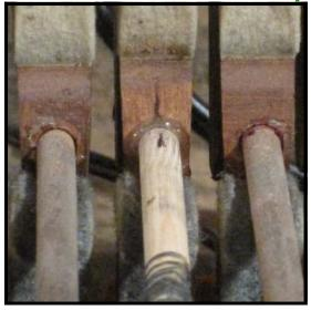
**Step 47:** Quickly place the assembled hammer shank / hammer into place and make any final adjustments in alignment. (Here's where you will appreciate the fact that the shank doesn't ratchet as you turn it.)
