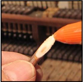
Step 10: Apply Titebond to one half of the joint. Be generous in your application, in that a little squeeze-out is helpful, unless you intend to remove the thread after the glue dries (refer ahead to page 16 for a note on this). Have your spool of thread within easy reaching distance at this point with a foot or so of thread unwound.
