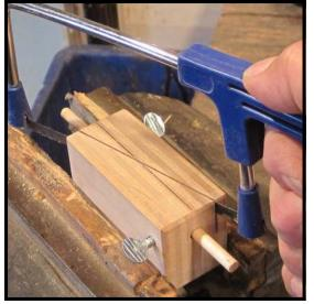
**Step 9:** Taking a new hammer shank, insert it into the miter box for cutting. Unless an extra long segment of shank is needed for a splice close to the flange, you can usually cut the shank at its center to produce two splicing shanks for use.
