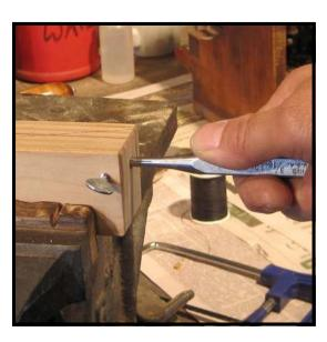
Caution: Before proceeding any further, clear out the hole in the miter box. If the left over stub doesn't fall out, use a blunt ended punch to tap it out. If you forget this step, you'll likely have a "log jam" develop at some point, when the split end of a shank, and the tapered end of a sawed off shank get jammed together. If this happens, you'll most likely need to drill the hole out again.
