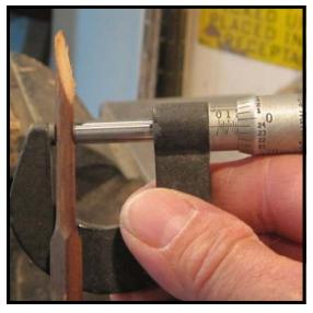
Step 8: Use a micrometer (Cat. No 3338 shown) to measure the diameter of the original shank. You will want to use a hammer shank that is at least as large as the original for splicing. In most cases upright shanks, (Cat. No. 504) which are 7/32 inch (or .2185") will be the best choice. Modern grand shanks typically measure either .204 or .196 inch. The slightly larger upright shank may be knurled or reduced to fit in a grand hammer that is bored for a standard grand shank.
