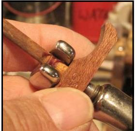
**Step 31:** As you turn the screw of the press down, you should feel the shank give way and begin to move. Watch underneath the hammer for evidence of the old shank emerging from the hammer head. On an old hammer and shank, the emerging shank will be lighter in color.
