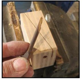
Notice that the extreme angle of the cut affords a large gluing area. With this amount of contact surface, a glue joint that will be as strong as an intact shank will be possible.
