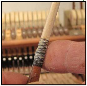
**Step 25:** Even the glue out over the windings by turning the shank and holding your finger stationary. Once dry, the windings will be anchored in place, maintaining a firm grip on the splice.
