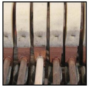
**Step 50:** With the splice successfully completed, the hammer / shank assembly may be returned to the action. The backcheck should be returned to its normal position. Soon, all the hammers will be functioning again.
