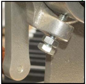
Note: Setting the amount of compression on the tool is a simple adjustment, as shown in the photo at left. The desired length of the knurl may also be easily adjusted. The hammer shank knurler may be attached permanently to your bench, or may be attached to a wood block to fit in a bench vise.
