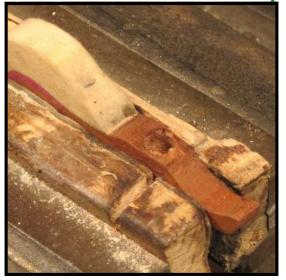
**Step 36:** To prepare the hammer for gluing, mount the hammer head in your vise with the bottom of the molding facing up.
