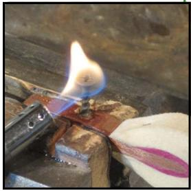
Step 32: If using the grand shank press doesn't budge the broken stub, try drilling a small pilot hole in the old shank, moistening it, then screwing in a dry-wall screw. Heat the screw as shown, then carefully pull out the stub of the shank with pliers. If all else fails, the remaining cylinder of wood may be removed in bits and pieces, or as a last resort the hole may be redrilled on a drill press.
