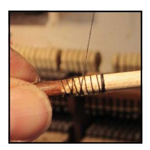
**Step 17:** When the winding is slightly beyond the extent of the splice begin wrapping away from your fingers again, maintaining or even widening the width of the windings. Continue back across the starting point, towards the hammer end of the splice.
