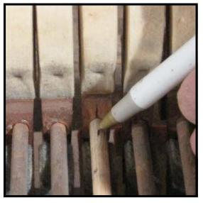
Step 41: Now, mark a line on the shank corresponding to the reference line on the bottom of the molding of the hammer head. Mark the line on the shank out far enough from the hammer so that it won't be obscured by the collar of glue which will be formed. This line will be sanded off once the glue has dried.
