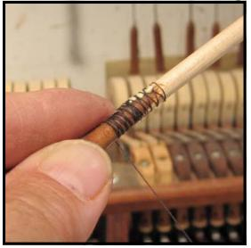
**Step 19:** Once you're to the end of the splice, hold the two ends of the thread firmly in place with the forefinger of your left hand (one thread not visible in photo), set the spool down on the bench, and pick up your scissors.
