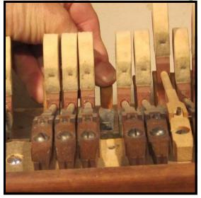
**Step 39:** In the spot where the repaired shank / hammer is going, temporarily push the backcheck further back to avoid contact with the extra bit of shank which will protrude from the top of the hammer until the glue has dried.
