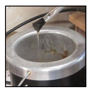
Hint: Check your glue before applying to the shank and hammer head. It should be fairly runny (but not watery), with the no evidence of unmelted crystals in the mix. Add a bit of water, or a few more crystals to obtain the correct consistency as needed. Allow a few more minutes to come back up to correct temperature, or for new crystals to melt..
