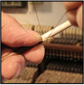
Step 15: Start your winding by wrapping the thread up and over the splice just above where you are pinching it the two halves of the splice together. Make three tight windings going in the direction away from your left hand.
