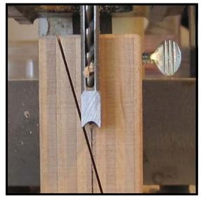
To solve this problem, a square hole on one end of the miter box may be cut with a mortising machine using a 1/4" mortising chisel bit. Before drilling the square hole, set the mortising machine's depth gauge so that the chisel bit will stop slightly before the diagonal guide line for the miter saw is reached, as shown in the photo. The hammer shank will then have a round hole supporting it on both sides of the saw, keeping it steady in the hole as it is being cut.
