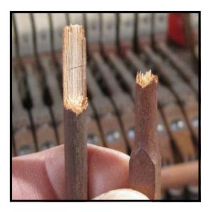
A long break compared to a stubby one. The long break presents adequate surface area for effective gluing and may be repaired using the same gluing and wrapping procedures as a prepared splice, but without having to add in a segment of new shank. For repairing this type a break, skip ahead to step 10.
