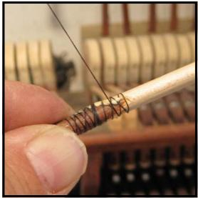
**Step 18:** Double back one last time, and head all the way to the flange end of the splice.
