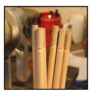
Note: Using the hammer shank knurler results in an evenness of results that is hard to achieve with the file rolling technique. It is especially useful on complete hammer replacement jobs, where every shank needs to be accurately knurled.
