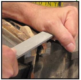
**Step 49:** Use a coarse, then fine file to mill down the top of the excess hammer shank.
