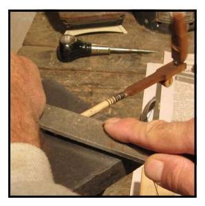
Step 35a: A light knurling of the shank may be accomplished by rolling the end of the shank several times at pressure under a flat bastard, coarse cut file (Cat. No. 252). For best results, use a solid metal surface, such as the anvil of a vise (shown), and position the flange off to the side so that it may rotate freely. Check the fit frequently, in that you don't want to go too far and end up with a loose fit.
