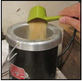
Step 33: If you intend to use hot animal hide glue in the process, now would be a good time to prepare the glue. I would recommend the Hold-Heet Electric Glue Pot (Cat. No. G-1155), used along with dry cabinet glue (Cat. No. 399-1/2). For this type of job, you only need to prepare a very small batch. Simply mix the glue crystals with water, and plug the pot in. Stir occasionally to maintain an even consistency.
