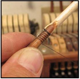
Step 16: With the initial windings done, double back, and begin heading towards the flanged end of the shank. As you do this, release your grip on the end of the thread with your teeth and allow that portion of the thread to fall loose. Scoot your fingers back a bit out of the way as you go, and wrap with a more widely spaced winding towards the flange end of the splice.
