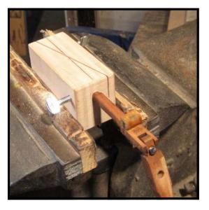
Note: Sooner than later you'll run into this problem. A break too close to the squared-off portion of the shank to fit far enough into the miter box to cut. You are literally trying to fit a square peg into a round hole. It doesn't work.
