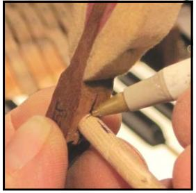
**Step 42:** Remove the shank and hammer, and mark one last reference line parallel to the underside of the molding of the hammer to watch as the shank is inserted into the hammer.
