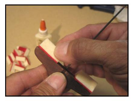
Once the damper heads and guide wires have been attended to, new damper felts will be glued in place, usually at the piano. High quality, precut damper felts are available for many grands. At other times, felt may be cut from strips so that the length of the dampers is precisely fitted to the damper heads.
