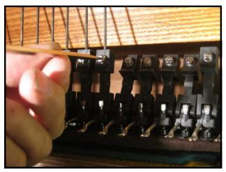
To access and remove the damper assemblies, the case will need to be disassembled to the extent that the action and keys may be drawn out of the piano. After removing the action from the piano, each damper will be taken out in order by loosening the set screw which holds the damper wire in place.
