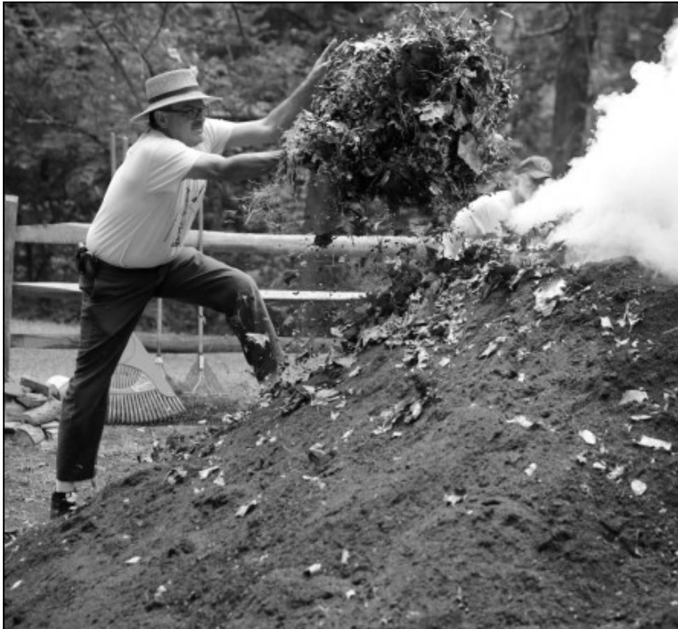
Cory Putt, Assistant Master Collier at Hopewell Furnace, and Friends board member, tends to the “pile” during the weeks long process of converting hardwoods, to charcoal, a very pure form of carbon. This fuel would be the source of intense heat during the iron making process. Cory will share insights of the process at the Friends Annual Business Meeting and Dinner.
