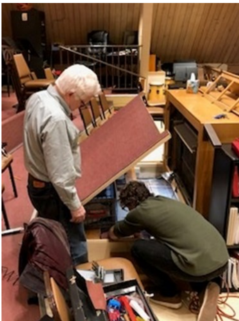
Two technicians from Bond Organ Builders, Inc. work to repair a broken solder in the pedal division.
