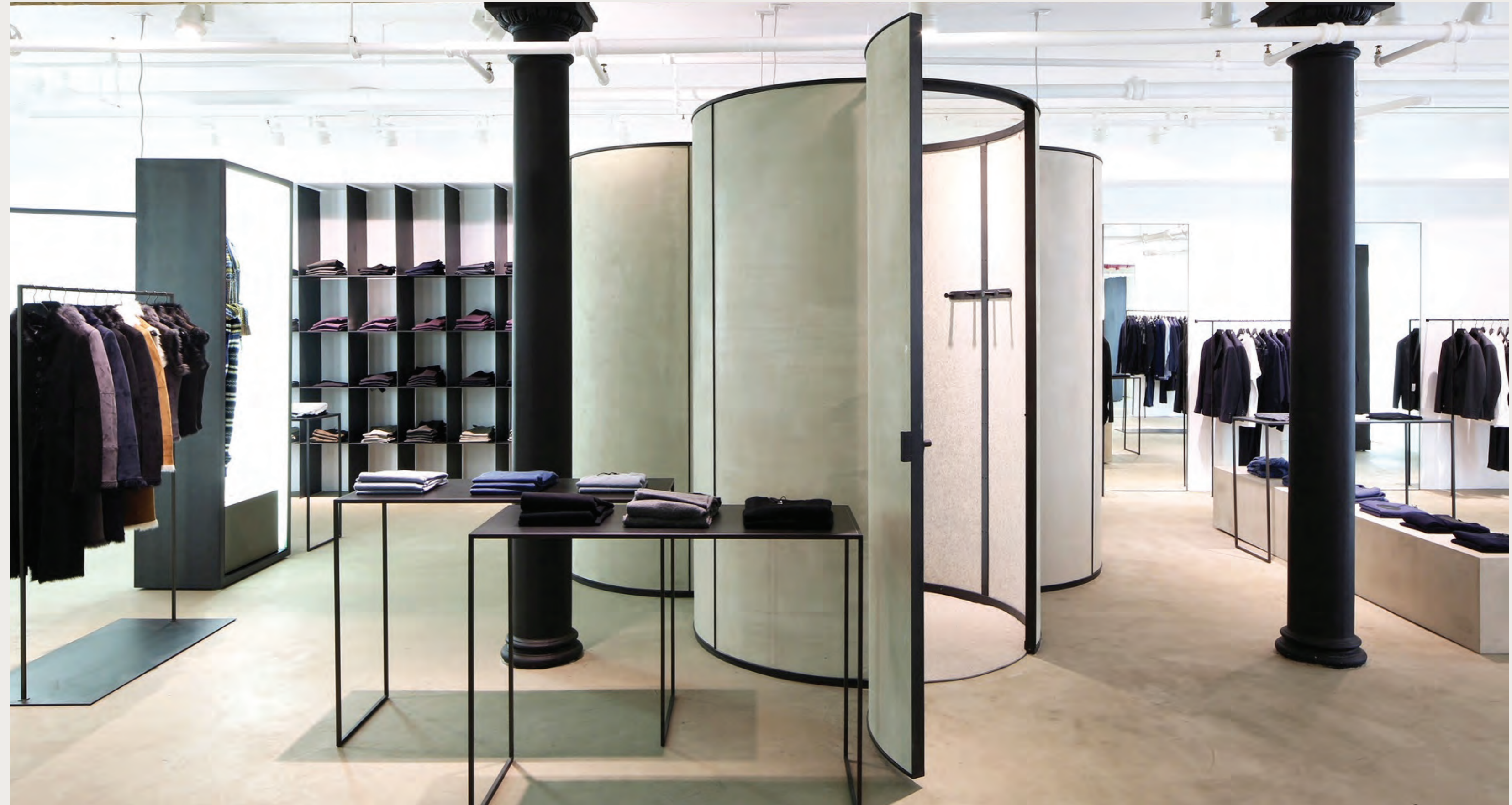
Steel, GFRC and felt lined freestanding changing rooms, freestanding steel furniture
