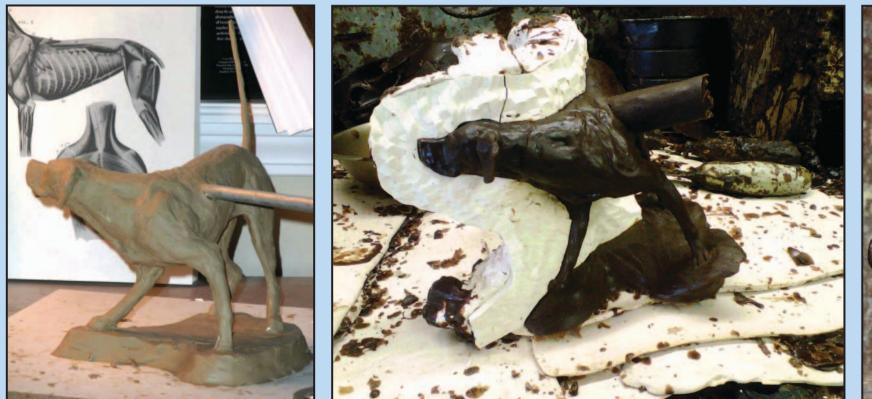
Three steps in the lost-wax process for casting the sculpture "Good Brakes" in bronze (from left): the original work in clay; a wax casting in its mold; and the finished product in bronze—one of 25 in a limited edition getting the final touches of a rich patina finish in the studio.
