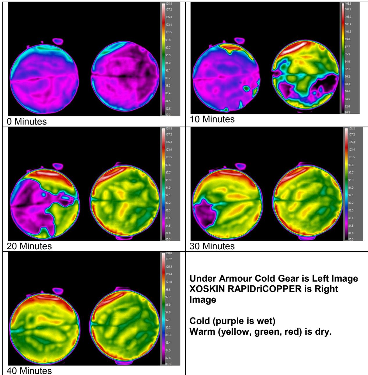
The XOSKIN garment achieves a stable temperature in less than 20 minutes. The UA Cold Gear garment requires an additional 20 minutes to achieve stable temperatures.
