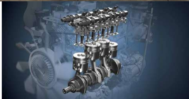
Diamond-like Carbon-coated Pistons and Injectors
