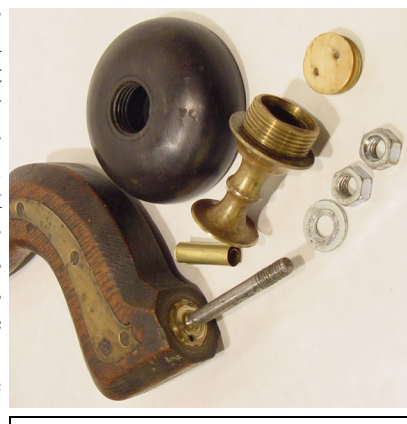
English brace head disassembled. It is held on with modern galvanized nuts and washer.
