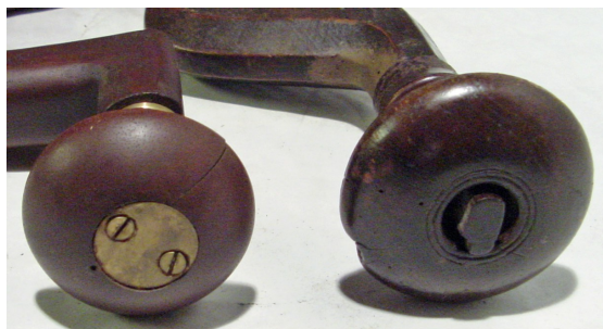
The authentic brace head to the right shows 150+ years of ageing where the repro head on the left shows none.
