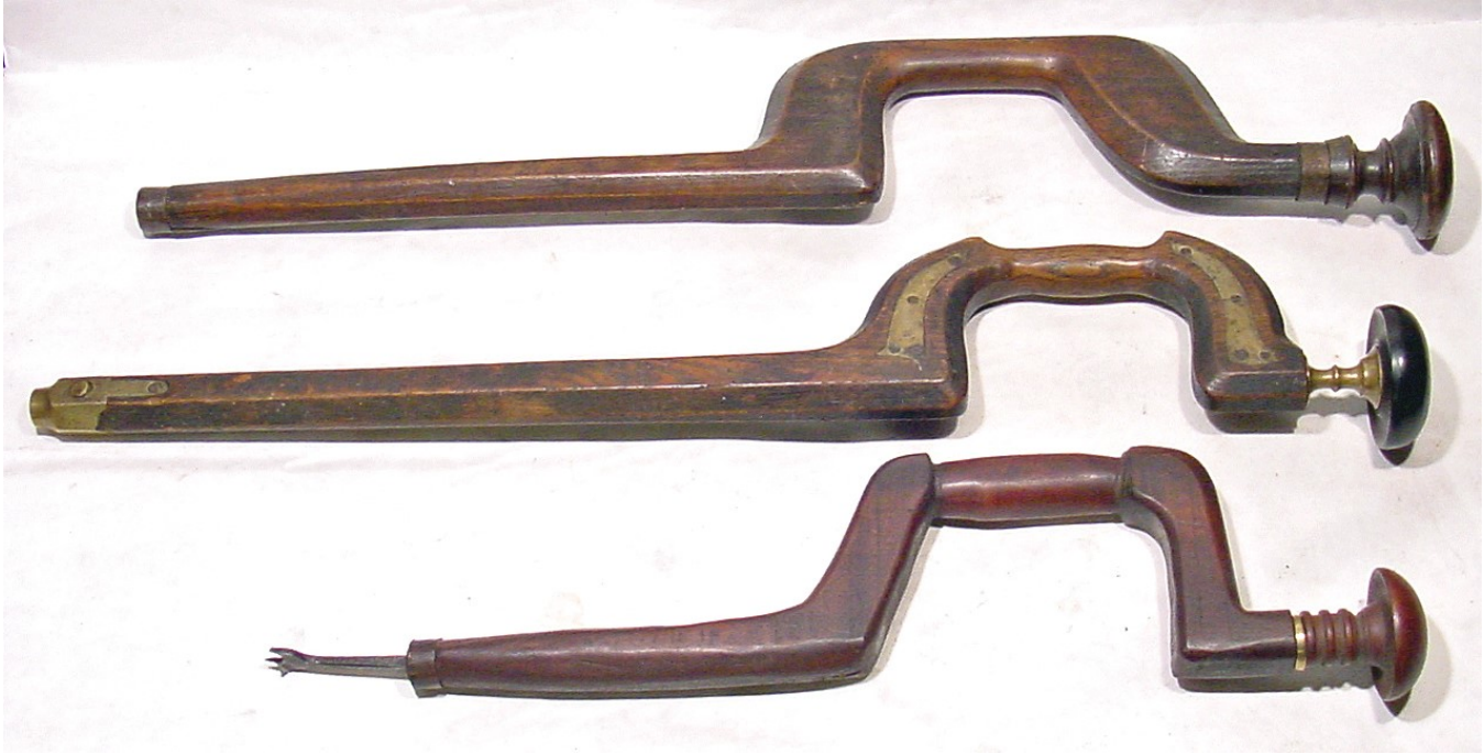
Three long shaft braces. The top is 100% authentic while the middle one is an antique craftsman made Sheffield style with a reworked neck and head. The bottom is a modern reproduction.
