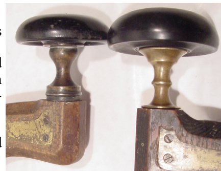
The English brace on the right lacks the brass bottom plate and washer under the neck that a typical Sheffield brace on the left has.
