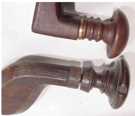
The lower authentic brace shows wear and well worn iron ferrules. The chip in the head has worn smooth over the years. Iron nails thru the upper web extension hold the head. The shiny brass in the top reproduction is a dead giveaway to newness.
