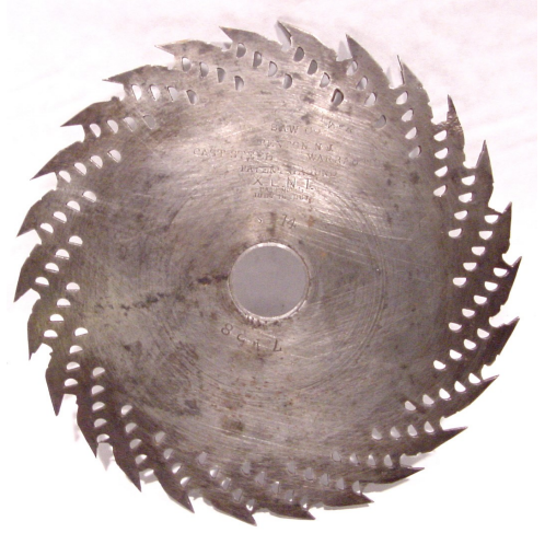
Circular saw blade with Emerson's patented perforations made by the American Saw Co.
