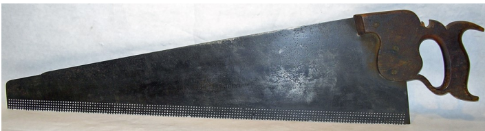
Above left is Emerson's 1866 patent for insertable teeth. Right is his first patent for perforated teeth. Below is a handsaw with similar perforated holes. It is etched "EMERSONS PATENT JULY 16, 1867. Below it is a close-up of the etch.
