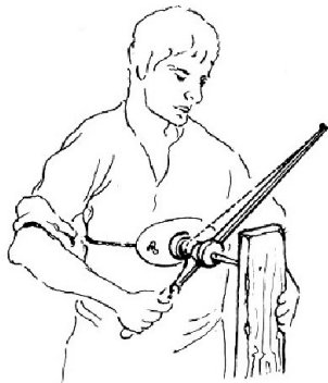
Bow drill with breast plate.
