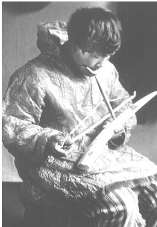
Inuit using bow drill with chin pressure to drill ivory.
