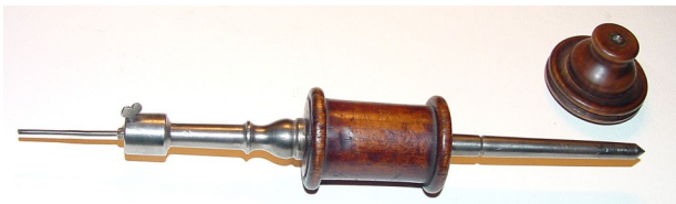
Simple bow drill with detached top which fits a point at the top of the metal spindle.
