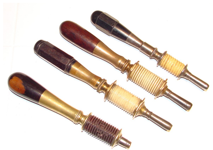
Above top is drill marked R. Fishley, made similar to NY style drills. Second drill is stamped N.E., NY (Napoleon Erlandsen). Third from top is marked HS & Co. (Hammacher & Schlemmer). Bottom is drill marked L. BRANDT, No. 220 1/2 5t St. N.Y. (See close-ups below).
