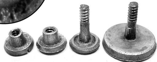
Disston patent No. 181648 given Aug. 29, 1876 for first generation of modern screw nuts used after the split nut design.
